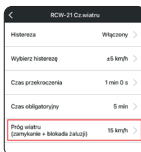
RCW-21 configuration screen (wind speed threshold setting when working with SFP-22)
